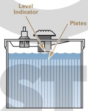
Maintain electrolyte level from at least 1/2-inch (13 mm) above plates to 1/4-inch (6 mm) below level indicator.
